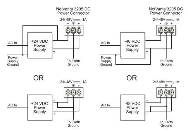
Figure 35. NetVanta 3205 DC Power Connection
